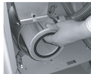
Dust collection filter cleaning
